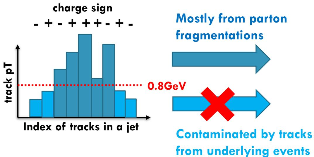
$$Q = \sum_{\text{all the tracks with } pT > 0.8 \text{ GeV}} \frac{\text{track } pT}{\text{jet } pT} \cdot \text{track charge}$$
