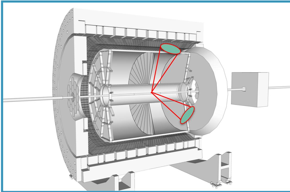
Can push to smaller  $x$  by using endcap calorimeter in forward region.
