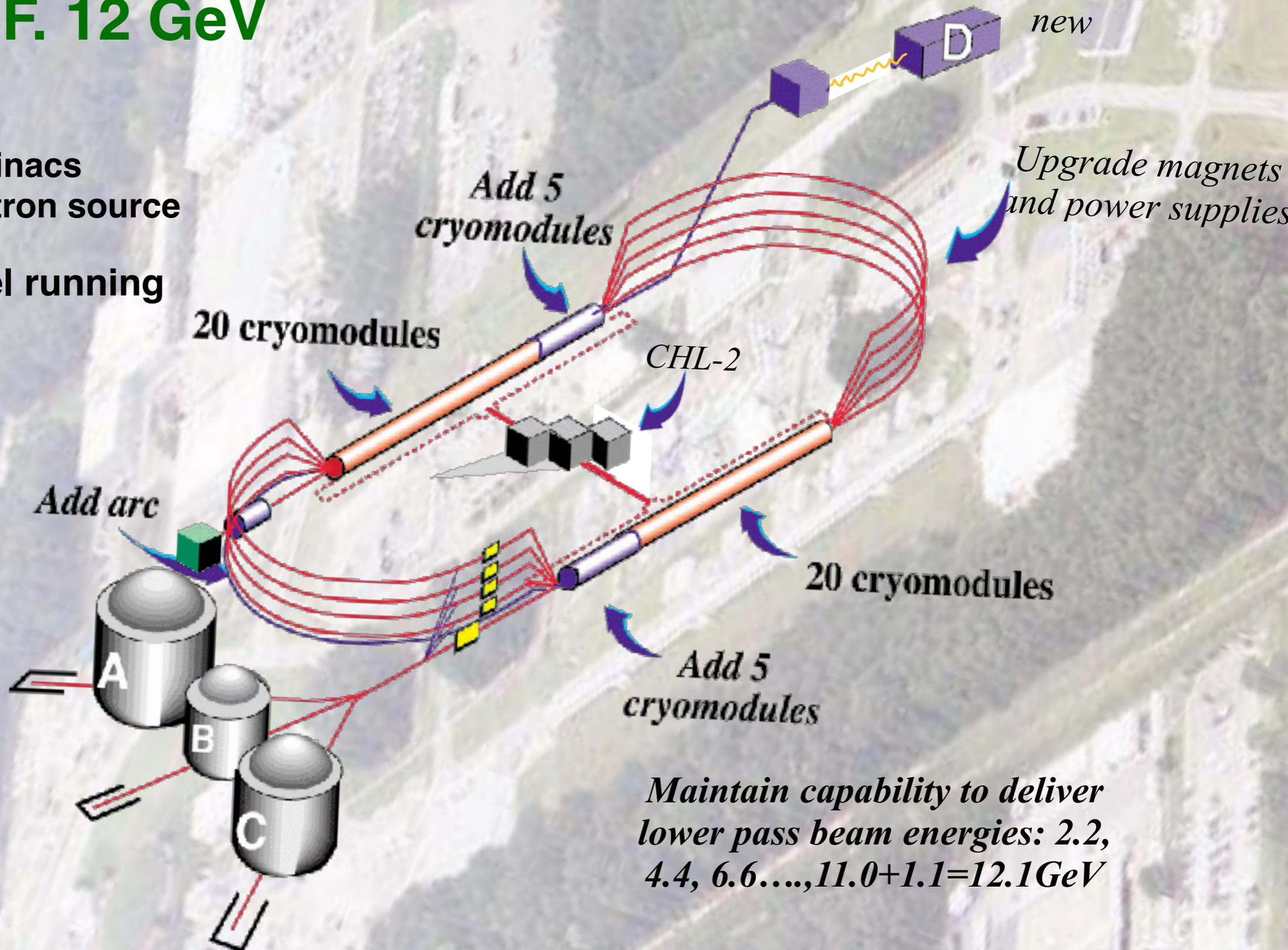
*Maintain capability to deliver lower pass beam energies: 2.2, 4.4, 6.6..., 11.0+1.1=12.1 GeV*
