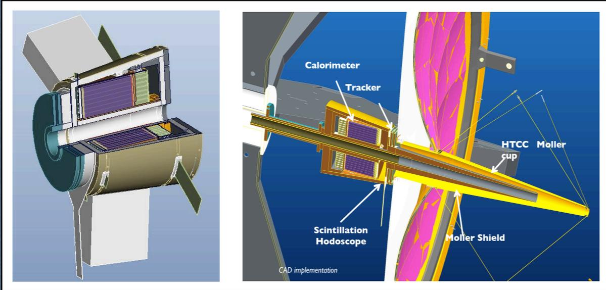
**FT-Cal:**  $\text{PbWO}_4$  calorimeter
