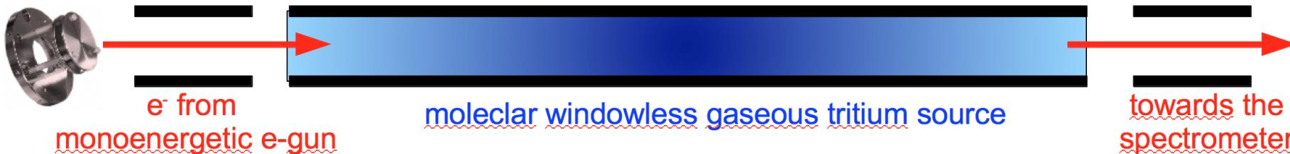
**Shooting electrons from monoenergetic pulsed UV-laser photoelectron source through tritium column density**
